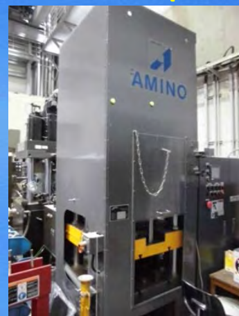
Hot Stretch Forming Test Machine
