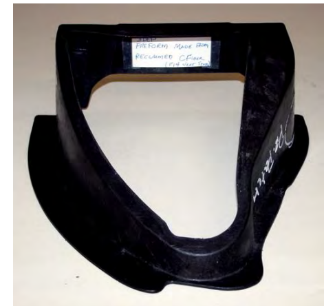
The finished part: A Chevrolet Corvette wheelhouse, made by Molded Fiber Glass Co Source: Materials Innovation Technologies
