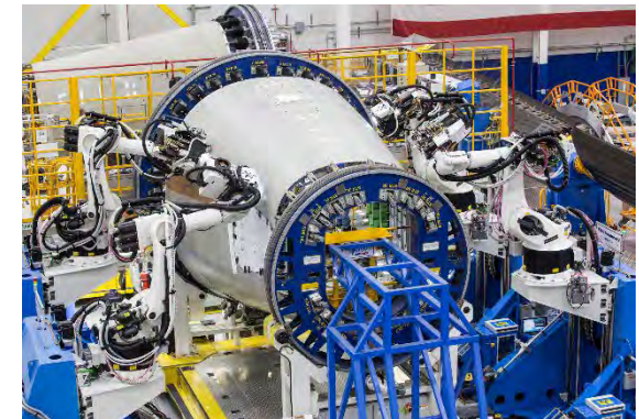
787 Aft Robotic Drill/Fill
