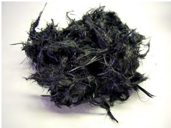
Reclaimed carbon fiber from an F-18 fiber's stabilator
