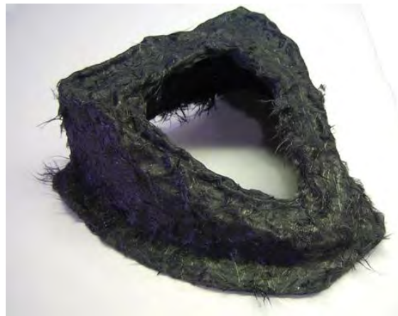
The preform, made from the F-18 recycle
