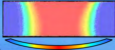
Example of strain distribution on a machined surface & Image of deformation seen from the side
