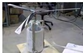
superconducting electric propulsion system
